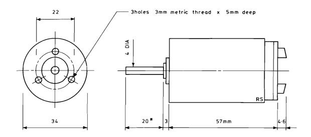
\* shaft length 6mm on type 222E motor
